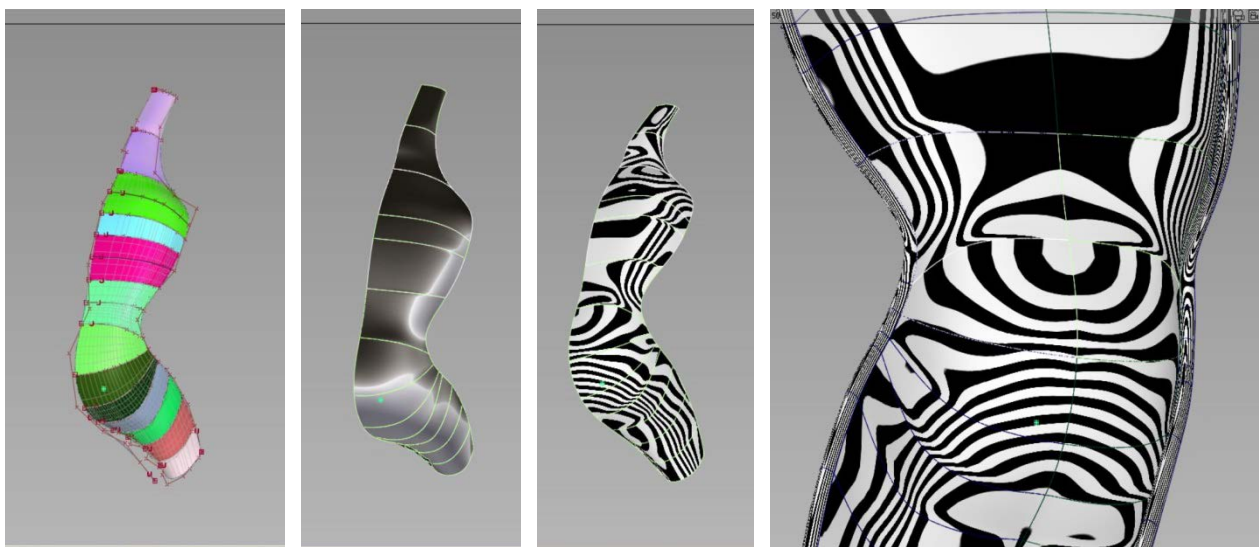
Figure 27 – Surfaces patches; analysed with various continuity analysis tools
